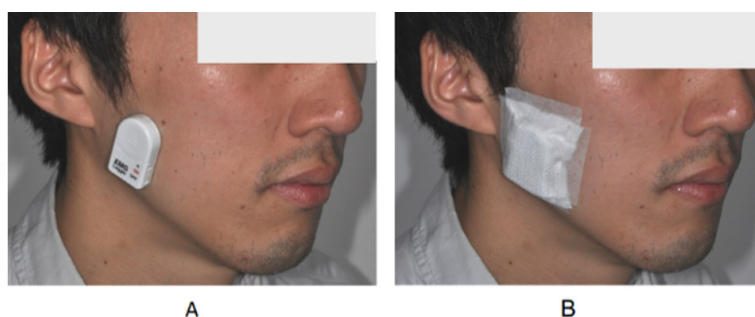
Fig. 3. FLA-500-SD attached to the skin surface with double-sided adhesive tape (A) and covered with a piece of gauze for camouflage (B) [5].
